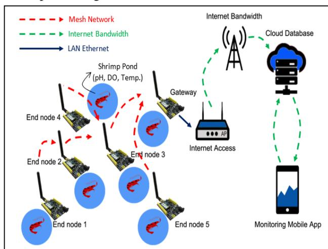
**Figure 2:** The Conceptual architecture of proposed SAM-IoT system in AQM environment
